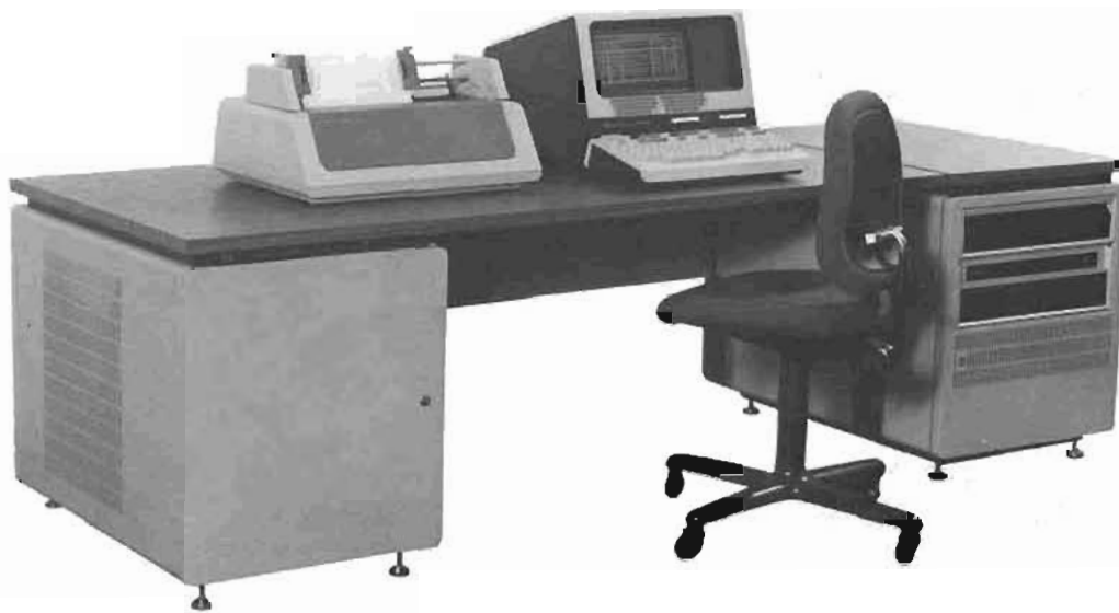
HP 1000 computer system (utilizing a 21MX controller and one or more HP 59310B interfaces)
